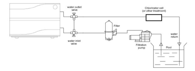
For optimum efficiency you may need to adjust the inlet and outlet valves to achieve a temperature differential of 2-3 degrees. Conducting a heat pump status check will verify the water inlet and outlet temperatures.
